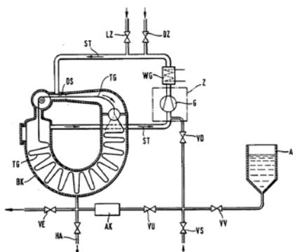
Figure 9. The jet dyeing machine. Picture from United States Patent US4862546
